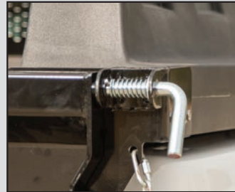
3/4" Diameter tailgate hitch pins
